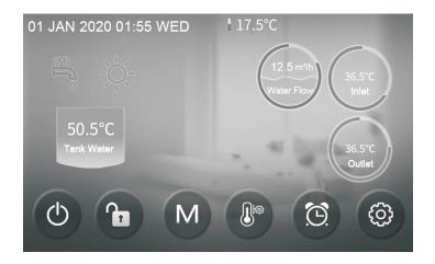
(2) Note: In starting up interface (on/off key is in red status), press the on/off key can shut down the machine.
