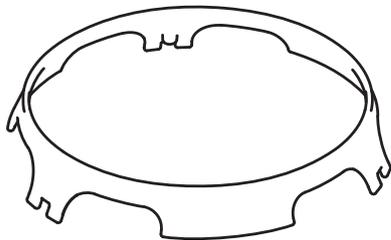
The wok cradle (**Fig. 2.8**) is designed to fit the centre burner. It will not fit any of the other burner pan supports.
