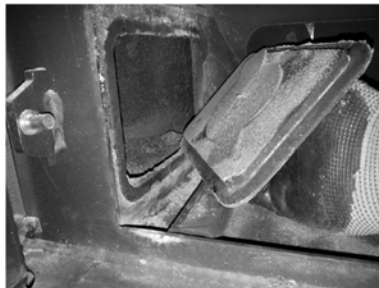
Figure 33 – Cleaning Vacuum the interior
