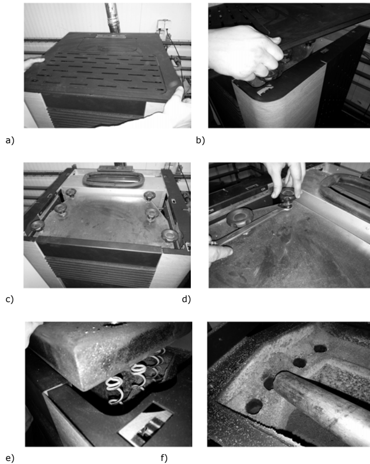
Figure 35 – Cleaning of gas passageways and turbulators
