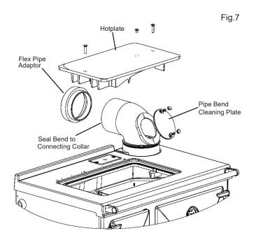
IT IS NOT RECOMMENDED TO CONNECT TO A FLUE SMALLER THAN 150mm (6") OR IN EXCESS OF 175mm (7") DIAMETER. 150mm (6") Diameter Flue Liner
