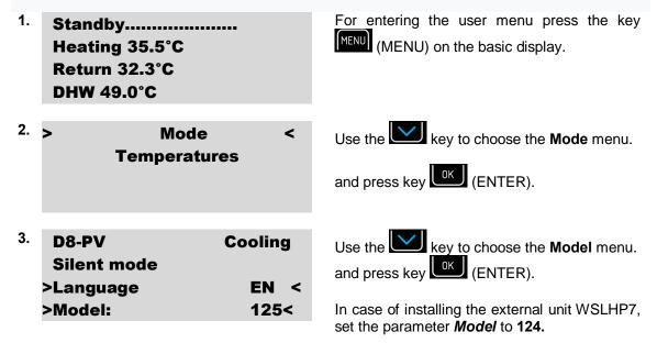
In case of installing the external unit WSLHP12, set the parameter *Model* to **125**.
