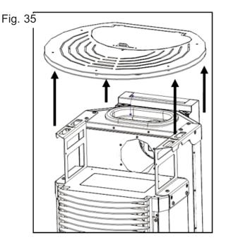
Place the upper front as shown in the opicture below, the flaps of the upper front must go inside the frame of the stove.
