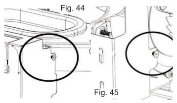
See figure below to show slot in side panel where screw should pass through the wide part before securing in the narrow section of the slot when the side panel is dropped into place
