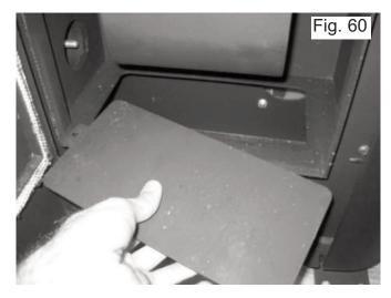
When the area is cleaned replace the trapdoor making sure it is seated correctly.
