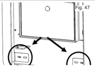
Figure above shows tabs overlapping the combustion chamber.
