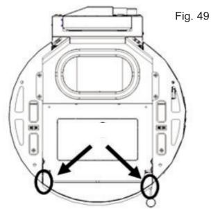
Fix the upper front to the stove using 4 additional screws adjacent to the 2 already fitted which can now be tigntened also. Fix the side panels in place using the 2 remaining screws.
