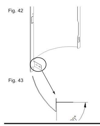
Place the covers on to the stove so that the screw on the back of the unit pass through the wide part of the key shaped slot, slide the panel down so that it is retained. See images below of scres side panels should be slotted onto.
