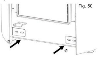
Make sure there is adeaquate space to fit the door. Replace the door using reverse of method to remove it, then adjust side panels to get an equal gap between the side panels and the door as per diagram below.
