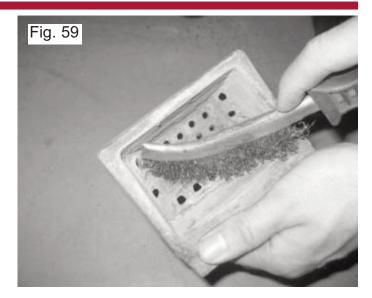
Put the burnpot back in place, making sure that it is seated properly, if the burnpot is seated incorrectly it will lead to problems during ignition or poor performance.
