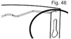
When fitting the covers, check that the tabs on the bottom overlap the combustion chamber and that the upper parts rest on the structure of the equipment
