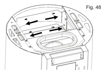
Make sure the side panels are aligned correctly with the upper front, in the locations as per picture below.
