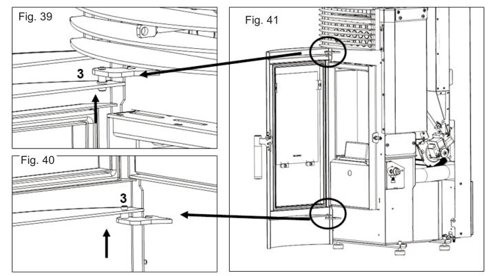
To fit the side panels it is necessary to remove the door from the stove, to remove the door, open the door first, lift the door to allow the bottom pin to disengage, move the door slightly to allow the door to drop without re-engaging the bottom pin then lower the door gently
