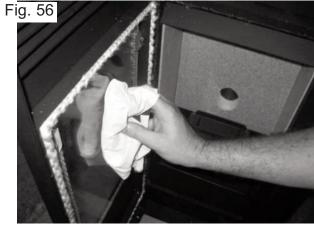
Fig.65 & 66 – Correct cleaning of the glass. Cleaning the glass:
