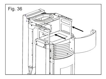
Screw the upper front to the frame using two of the screws provided. Place screws in the location shown below.Do not fully tighten as a small adjustment may be necessaary.
