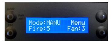
Auto mode: In this mode, the unit is turned on at maximum power until reaching a temperature 1°C above the selected temperature (set point temperature). After reaching the selected temperature, the unit switches to the minimum operating power. The set-point temperature can be set between 5 and 40°C by pressing the "-" key.
