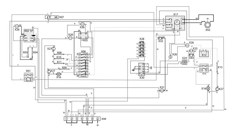
**Key**The connections shown in the circuit diagram are for single-phase. The ratings are for 230 V 50 Hz.
