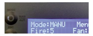
Auto mode: In this mode, the unit is turned on at maximum power until reaching a temperature 1°C above the selected temperature (set point temperature). After reaching the selected temperature, the unit switches to the minimum operating power. The set-point temperature can be set between 5 and 40°C by pressing the "-" key.
