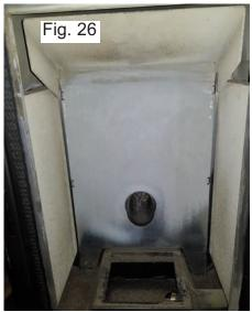
To remove the vermiculite lift the it with one hand and the baffle with the other, when both are raised move the vermiculite out over the tab at the bottom edge allowing the vermiculite then be removed. Then remove the flue baffle.
