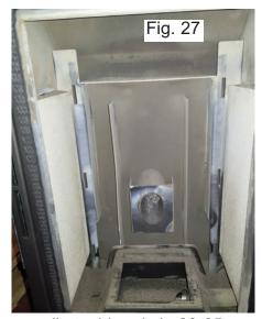
Using a small steel brush (a 20-25mm diameter steel brush) remove the ashes in the flue passageway that are difficult to access and the more ingrained ashes that are found in the walls of the combustion chamber. Use the vacuum cleaner to remove dirt from inside the combustion chamber. Replace the parts in reverse order.
