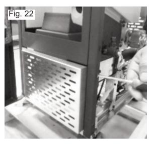
Once the covers have been removed, remove the side and front covers of the flue passageway.
