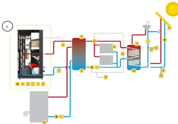
Figure 52 - Connection to central heating radiators with another boiler support and sanitary water combined with solar panel
