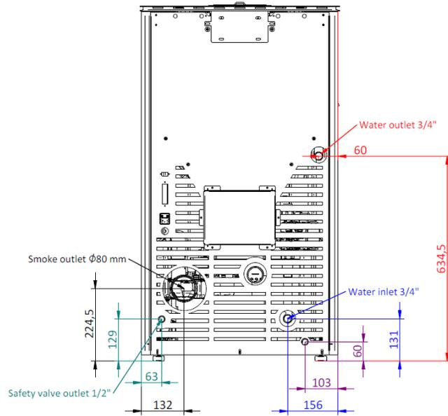
**Figure 5 - Hydraulic connections of the free-standing pellet fire unit K1200**
