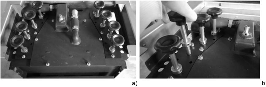
**Figure 36 - Cleaning the turbulators**
