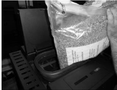
Figure 31 - Refilling the pellet reservoir
