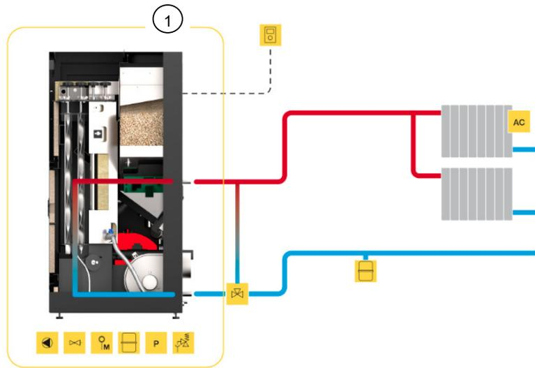
Figure 49 - Simple connection only the central heating radiators
