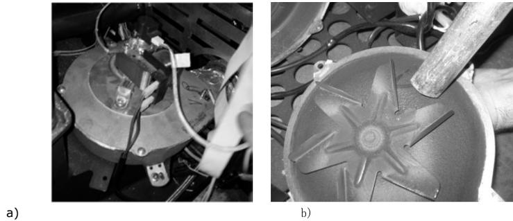
**Figure 42 - Cleaning Vacuum the interior**
