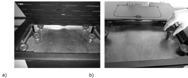
**Figure 33 - Cleaning the turbulators**
