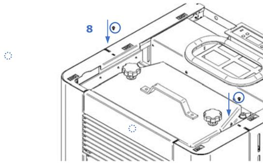
Figure 21 - Assembly of the casings K1200
