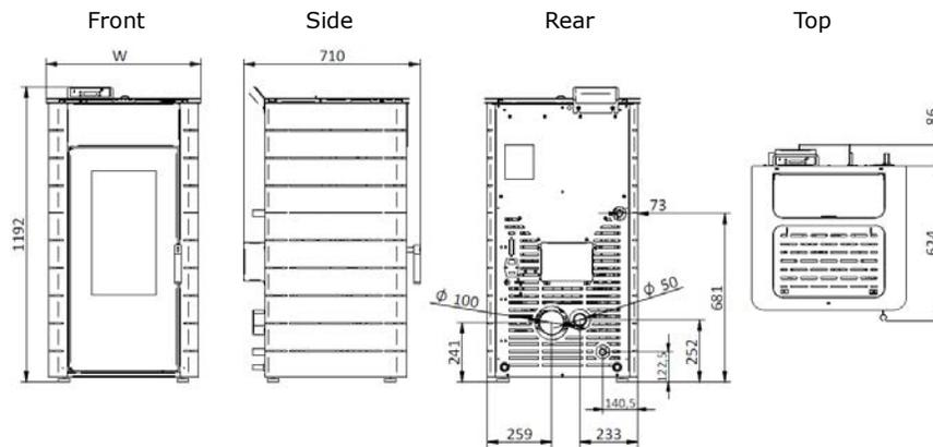
**Figure 3 - Dimensions of the free-standing pellet fire unit K1700 Table 2 - Dimensions of the free-standing pellet fire unit K1700**
