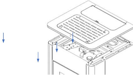
Figure 28 - Assembly of the casings K1700 and K2300
