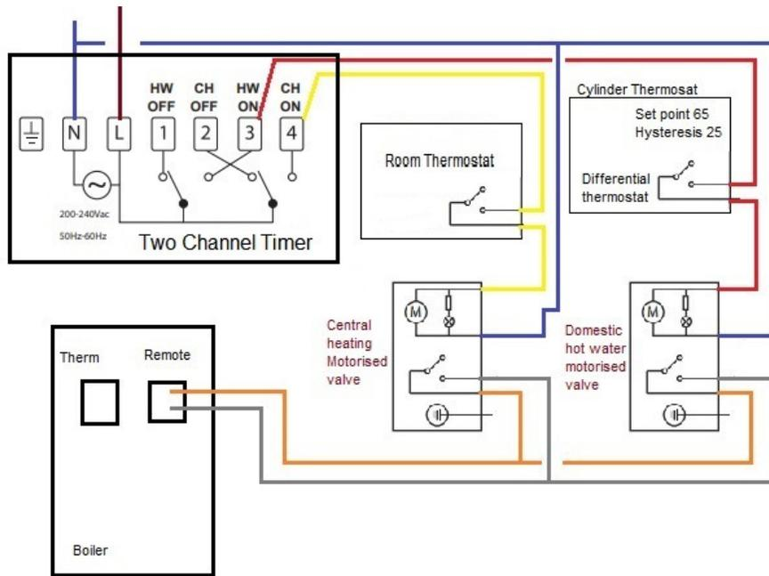
Figure 51 - Electrical connection of a thermostat (ambient air monitoring) of a differential thermostat connected to the domestic hot water and 2 way motorized valves
