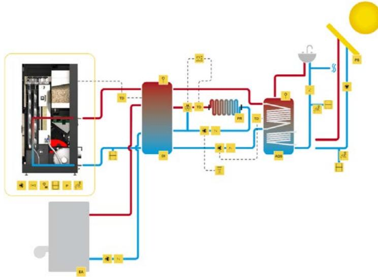
Figure 53 - Connecting underfloor heating in conjunction with another boiler support and sanitary water combined with solar panel
