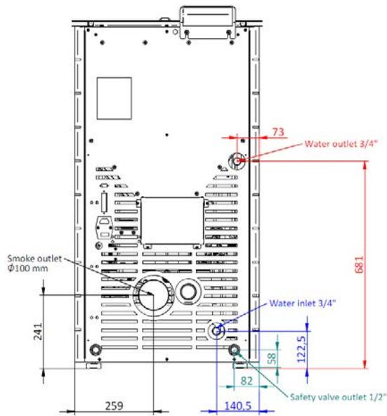
**Figure 6 - Hydraulic connections of the free-standing pellet fire unit K1700 (Flat)**
