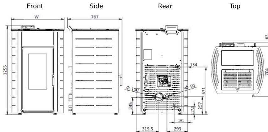
**Figure 4 - Dimensions of the free-standing pellet fire unit K2300**
