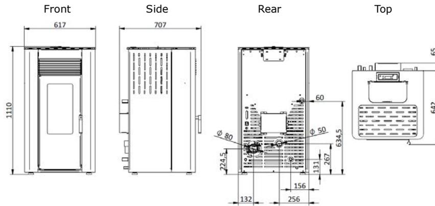
**Figure 2 - Dimensions of the free-standing pellet fire unit K1200**
