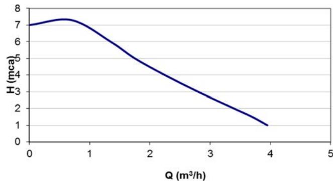
Figure 56 - Circulating pump performance graph
