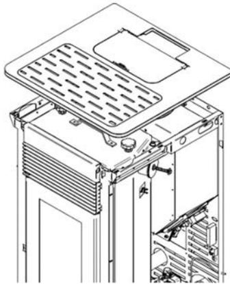
Figure 22 - Assembly of the casings K1200
