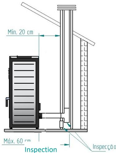
Figure 12 - Side view of the installation with a chimney, showing the inspection point
