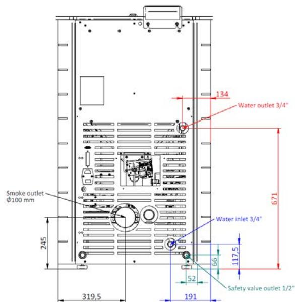
**Figure 7 - Hydraulic connections of the free-standing pellet fire unit K2300 (curved)**
