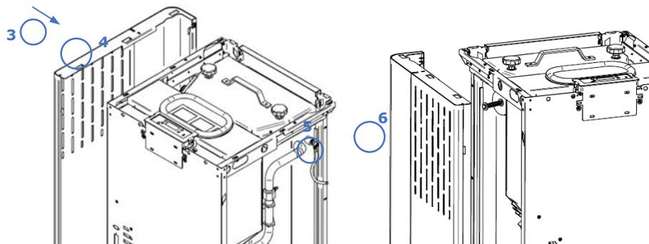
**Figure 19 - Assembly of the casings K1200**
