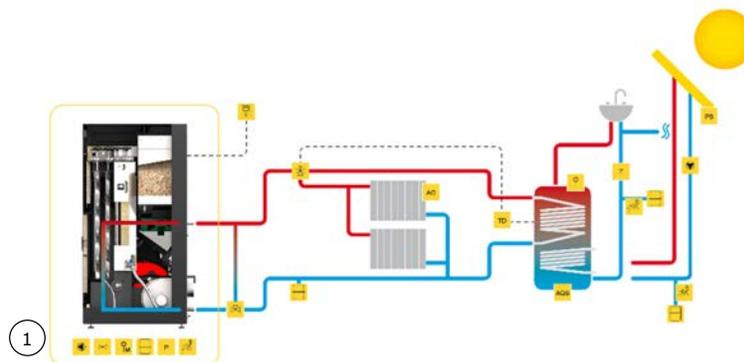
Figure 50 - Connection to central heating radiators and sanitary water combined with solar panel
