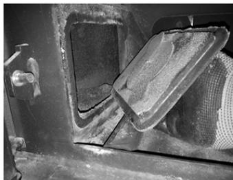
**Figure 41 - Cleaning Vacuum the interior**
