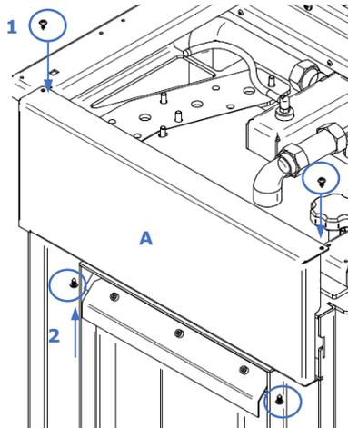
**Figure 25 - Fitting the front cover K1700 and K2300**
