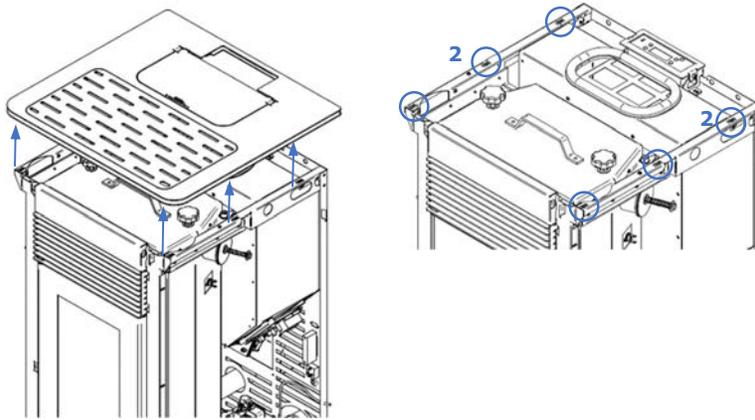
**Figure 17 - Removing the top K1200**
