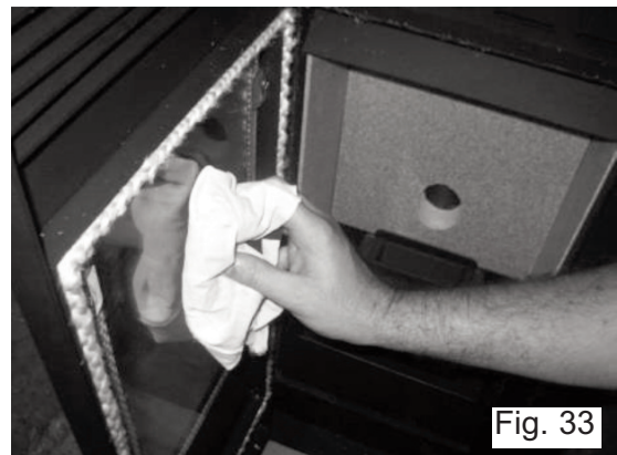
Fig.32 & 33 – Correct cleaning of the glass.
